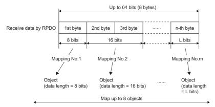
While the RJ71CN91 is operating, each RPDO can be stopped, configured, or started via the program or by other nodes by changing the object dictionary corresponding to the parameters.
