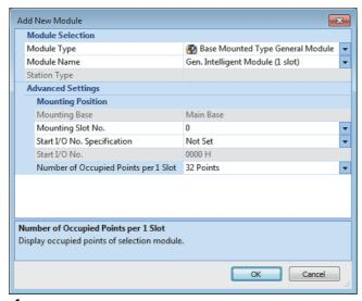
Write the set parameters to the CPU module, and reset the CPU module or power off and on the system.
